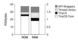
Figure 9. Breakdown of the binary code size and RAM usage of a complete TOSThreads kernel based on the standard C API compiled together with TinyLD.
