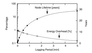
Figure 5. Energy overhead of implementing SSF application using TOSThreads as a function of the logging period. Also shown is the node lifetime, using standard AA batteries as the energy source.
