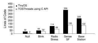
Figure 8. Comparison of application lines of code for five sample applications implemented using standard TinyOS and TOSThreads.
