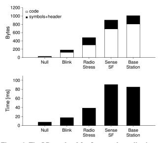
Figure 6. TinyLD overhead for five sample applications. The top graph shows the size of each application using the MicroExe format and the bottom graph presents the time TinyLD requires to link and load each application.
