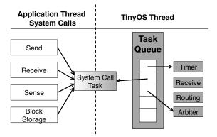
Figure 4. TOSThreads exposes kernel APIs through blocking system calls wrapped around event-driven TinyOS services. These wrappers (white boxes on the left) run their respective system calls inside a single shared TinyOS task. This task is interleaved with other TinyOS tasks (grey boxes on the right) which TinyOS itself posts.
