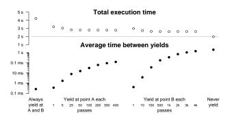
Figure 1. Total execution time and average time between yields of various yielding strategies for a compression algorithm applied on a set of 13 gray-scale images captured with the Cyclops platform.
