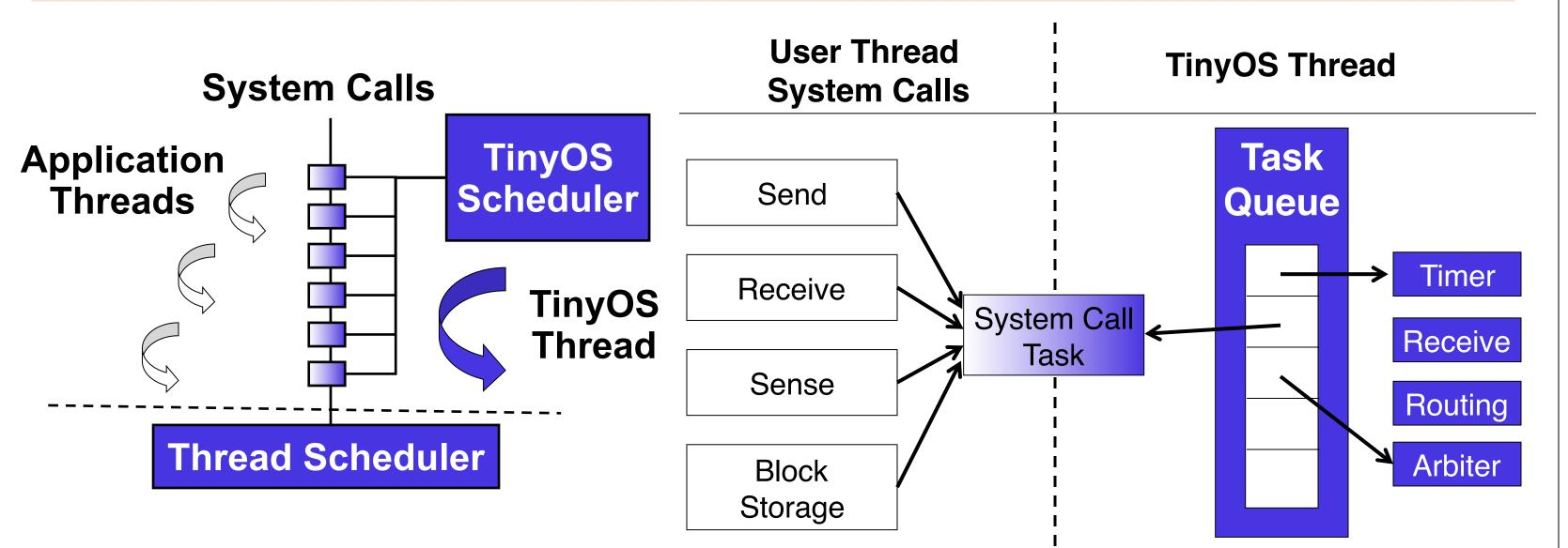
**TOSThreads** allows fully preemptive application threads to run concurrently, making blocking calls to a single higher priority TinyOS kernel thread. Message-passing threading model does not sacrifice the underlying TinyOS event-driven model.
