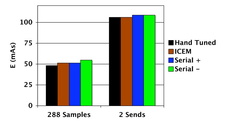
Application energy with 5 minute sampling interval and one send batch every 12 hours
