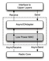
Figure 2. Asynchronous to synchronous I/O adaptation
