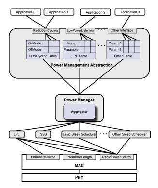
Figure 1. Radio Power Management Architecture
